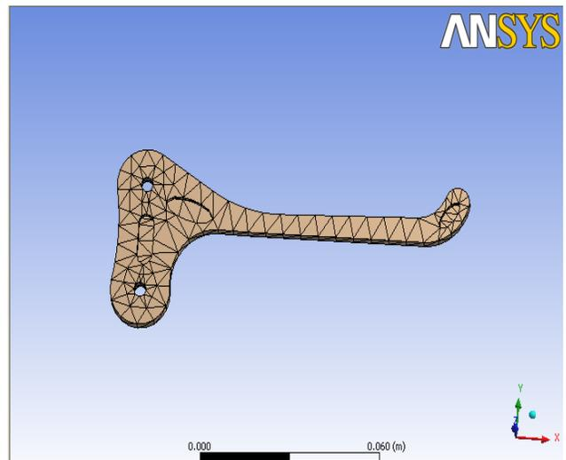
Figure 10. Shows the coarse meshing of modified brake lever model in Ansys workbench.
