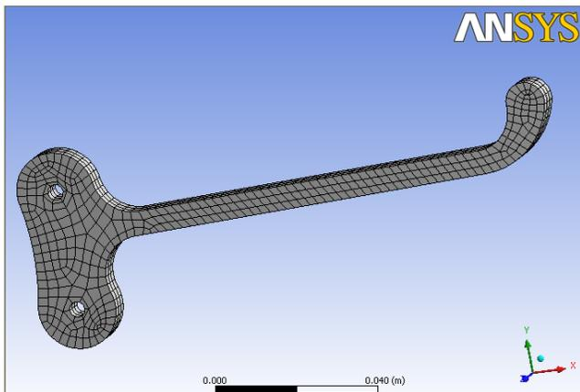
Figure 8. Shows the medium meshing of brake lever model in Ansys workbench.
