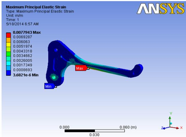
C. Comparison of simulation results of brake lever.
