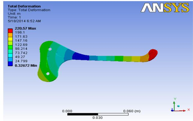
*B. Modified design of brake lever.*
