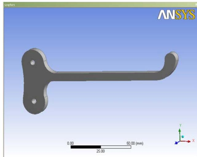
Figure 5. Shows the imported simple design of the brake lever in Ansys workbench.
