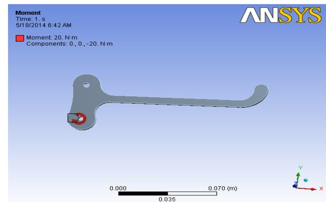
Figure 15. Applying the moment of 20 Nm.
