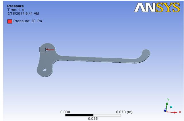
Figure 13. Applying the pressure of 20 Pa.
