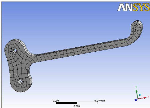
Figure 7. Shows the medium meshing of brake lever model in Ansys workbench.
