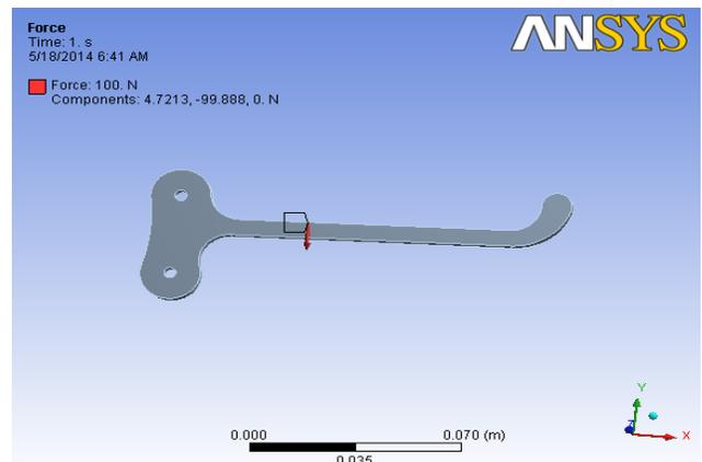
Figure 14. Applying the force of 100 N.
