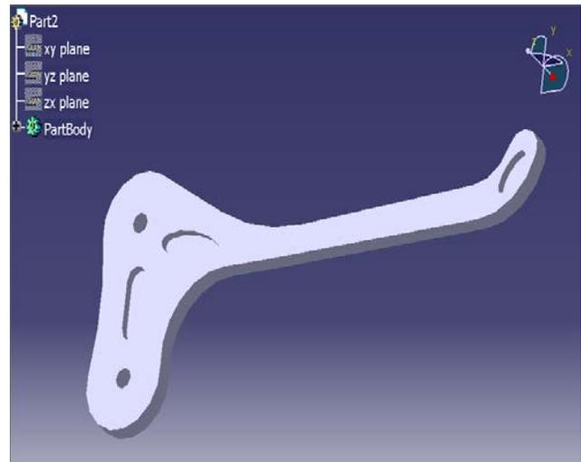
Figure 4. Shows modified design of the brake lever with 4mm thickness.
