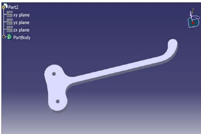
Figure 3. Shows the simple design of the brake lever with 6mm thickness.
