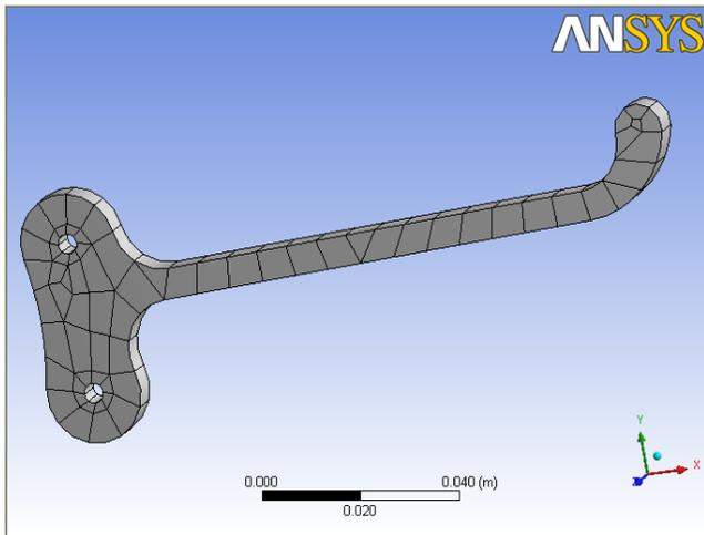
Figure 6. Shows the coarse meshing of brake lever model in Ansys workbench.
