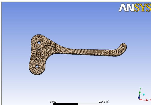
Figure 12. Shows the fine meshing of modified brake lever model in Ansys workbench.
