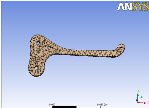
Figure 11. Shows the medium meshing of modified brake lever model in Ansys workbench.
