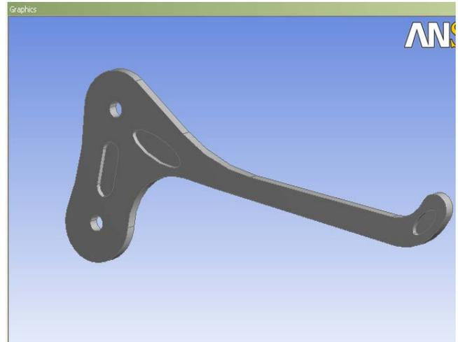
Figure 9. Shows the imported modified design of the brake lever in Ansys workbench.
