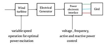
Figure 4: Variable speed wind energy conversion system
