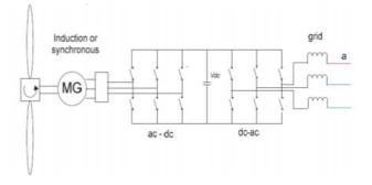
Figure 5: Fully variable wind energy conversion system
