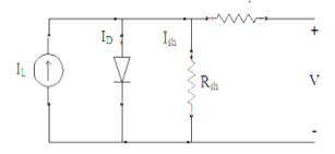
Figure 3: Equivalent Electrical Circuit of PVC
