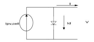
Figure 2: Show ideal photovoltaic cell equivalent circuit
