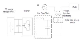
Figure 3: Basic structure of a conventional DVR
