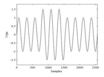
Figure 2: Voltage swell waveform
