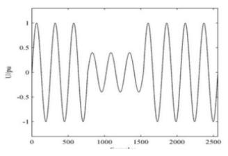
Figure 1: Voltage sag waveform
