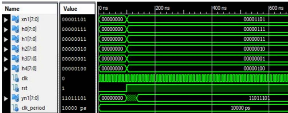
**Fig. 5:** Output Test Bench Waveform of Narrow Band Filter (Filter Coefficient N=5)
