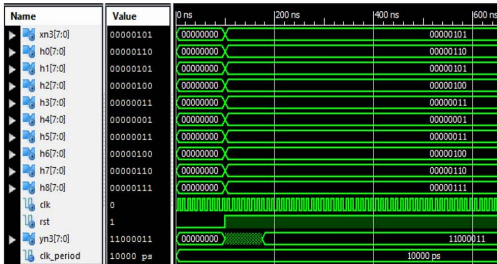
**Fig. 6:** Output Waveform of 9\_tap Narrow Band Filter
