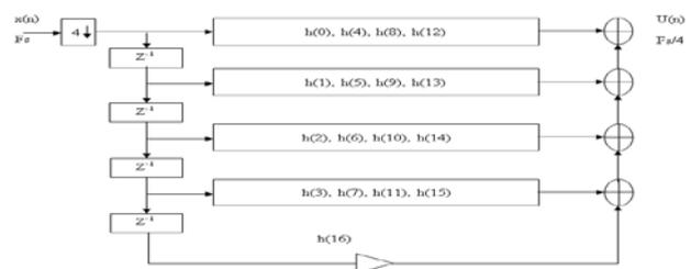
**Fig. 4:** Decimator structure with filter order  $N1=17$  and  $M=4$
