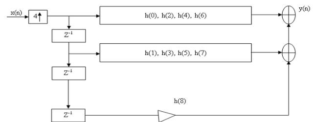
**Fig. 3:** Interpolator structure with filter order  $N3=9$  and  $L=4$
