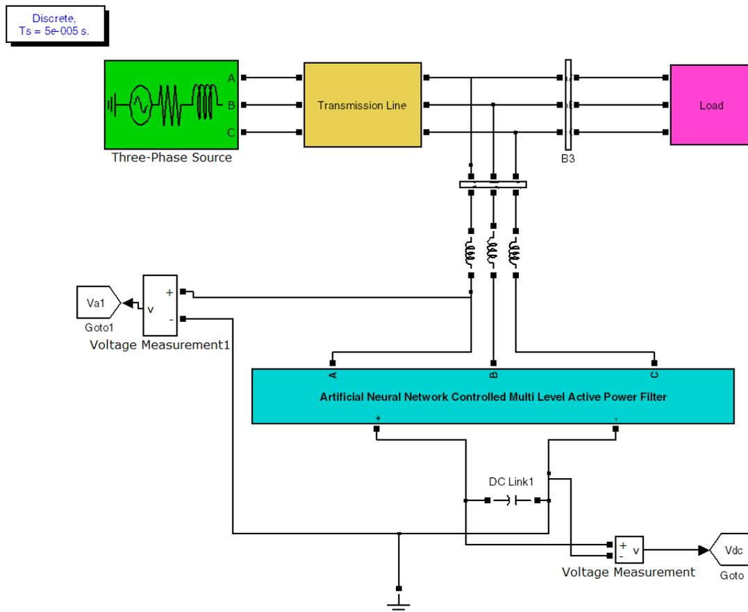
Figure 2.1 Simulink Model of Proposed work
