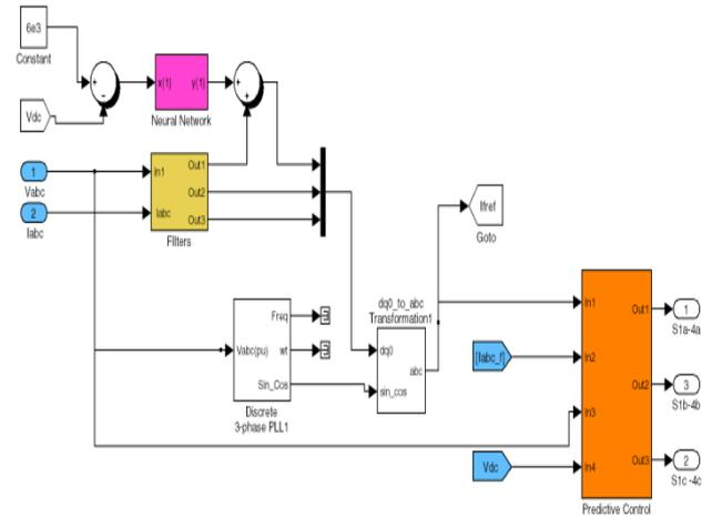
Fig.2.3 ANN based Controller Architecture
