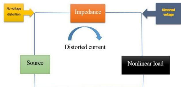
Figure 1.1 Flow of harmonic currents and generation of harmonic voltages.
