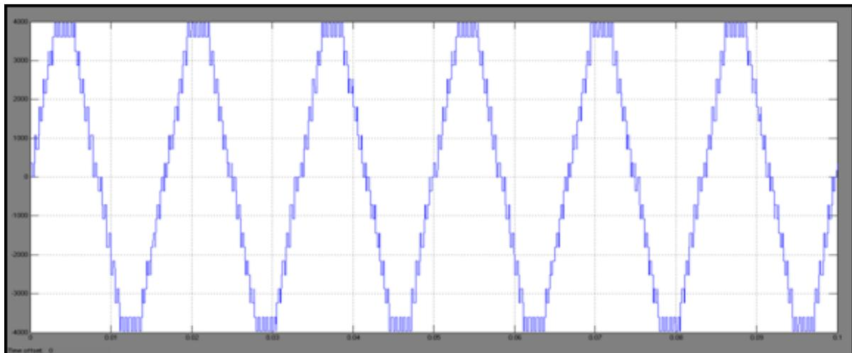
Figure 3.4 7 level active power filter outcome waveform.
