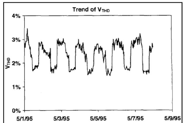
Fig. 1.4 Trend of Voltage Total Harmonic Distortion Demonstrating Daily Cycle for One Week
