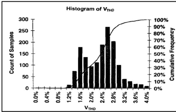
Fig. 1.5 Histogram of Voltage Total Harmonic Distortion for One Month Demonstrating Bimodal Distribution
