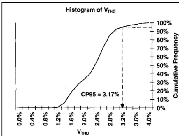
Fig. 1.6 Demonstration of Graphical Method of Calculating the CP95 of a Distribution
