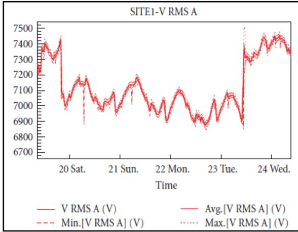
Fig. 1.2 Time trend of an RMS voltage in PQ analysis
