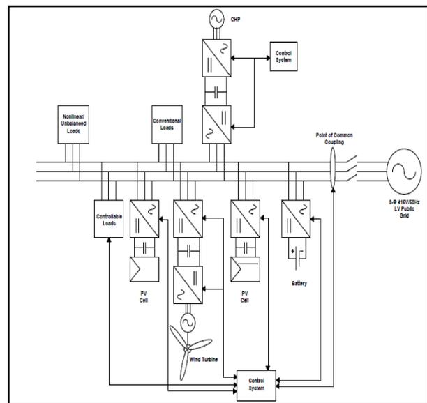
Fig. 1.1 Concept of a Microgrid
