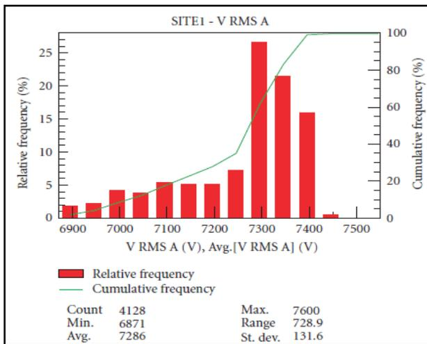
Fig. 1.3 Histogram representation of RMS voltage indicates the statistical distribution of the RMS voltage magnitude
