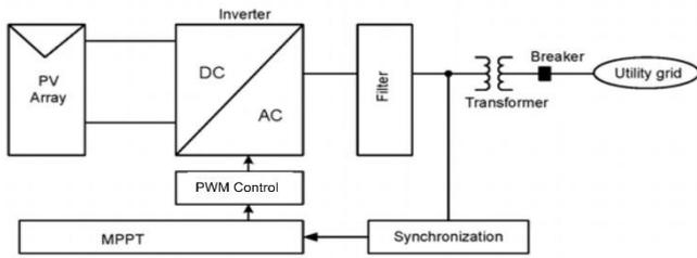
The output quantity of associate degree electrical converter (voltage in VSI and current in CSI) is beat and contains shift harmonics aboard a sixty Hertz central. Keeping in mind the tip goal to isolate the sixty Hertz half, a filter is basic at the AC terminal of the electrical converter, wherever it's interfaced to the grid.
