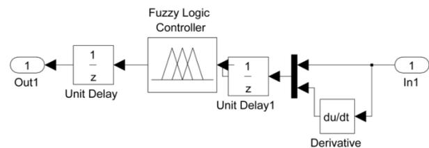
Figure 3.3 Fuzzy Controller in Simulink.
