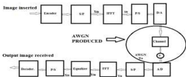
Fig.2.1 A typical OFDM transceiver system.
