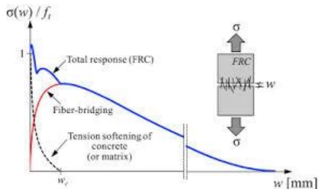
Fig. 1 Concrete The behavior of fiber reinforced concrete
