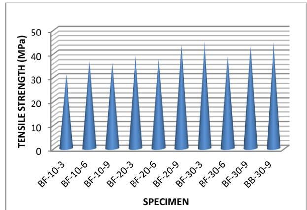
Figure 2: Basalt Bundles: Split tensile strength
