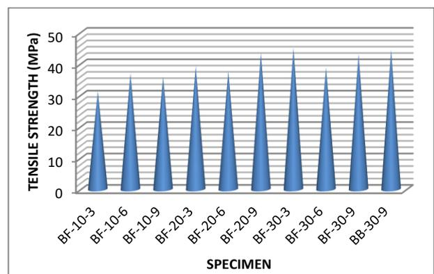
Figure 3: Basalt Bundles: Split tensile strength
