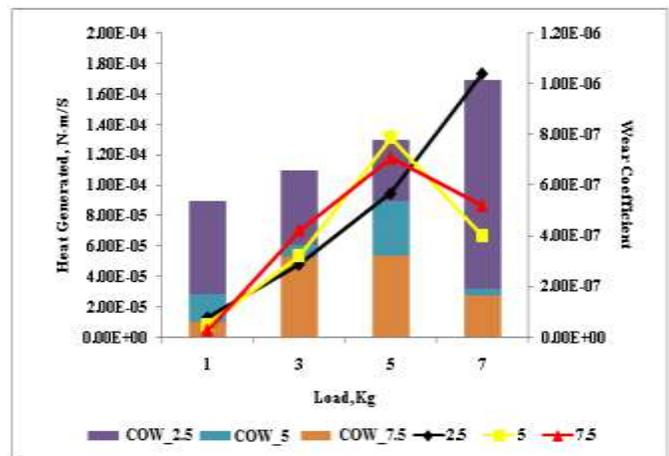
Fig. 5: Heat generated and COW as a function of applied load for a constant sliding distance of 1000 meters for 24 hours water absorbed ABS Samples
