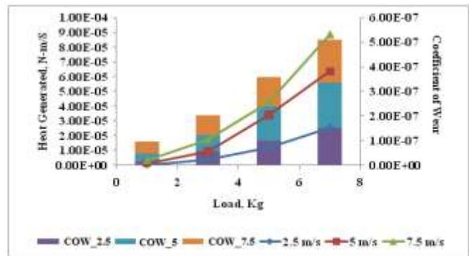
Fig. 8: Heat generated and COW as a function of applied load for a constant sliding distance of 1000 meters for electroplated ABS Samples
