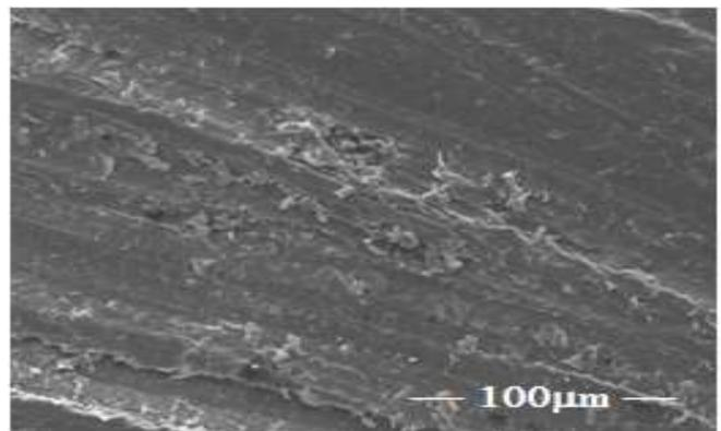
Fig. 9: SEM of Electroplated ABS sample subjected to applied load of 7 kg, sliding velocity of 5 m/s and sliding distance of 1000 m
