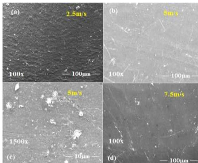
Fig. 3: SEM image of Normal ABS samples subjected to wear studies with an applied load of 7Kg and a sliding distance of 1000m with varying sliding velocity.
