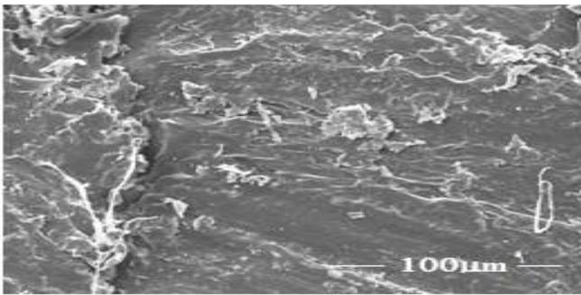
Fig. 6: SEM of 24 hours water absorbed ABS sample subjected to applied load of 7 kg, sliding velocity of 2.5 m/s and sliding distance of 1000 m
