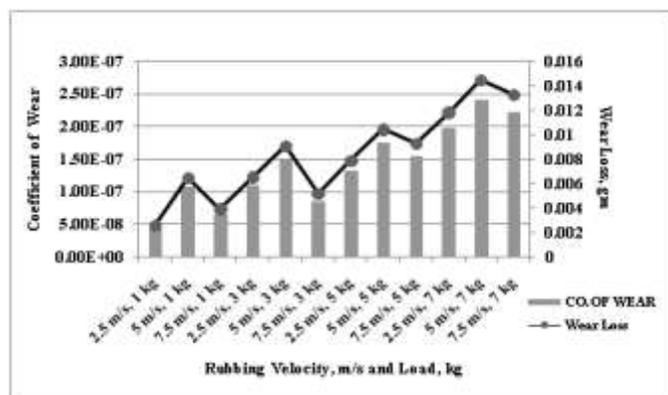
Fig. 2: Coefficient of wear and Wear loss as a function of Rubbing velocity and Load for a constant sliding distance of 1000 meters for Normal ABS Samples
