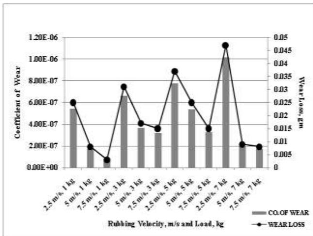
Fig. 4: Coefficient of wear and Wear loss as a function of Rubbing velocity and Load for a constant sliding distance of 1000 meters for 24 hours water absorbed ABS Samples
