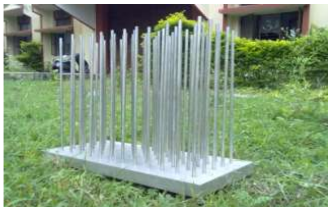
Fig. 2 Heat sink with circular fins
