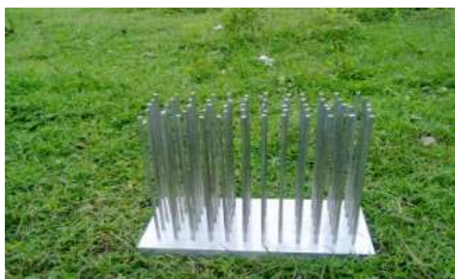
Fig.3 Heat sink with square fins
