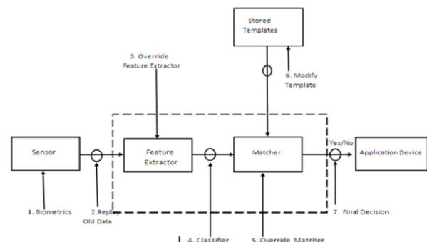
Figure 2.1: Process Logic Flow Diagram
