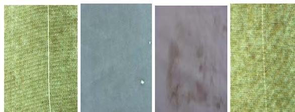
Fig. 2.1 Web Material with Missing yarn, Hole, Oil Spot and Needle Line
