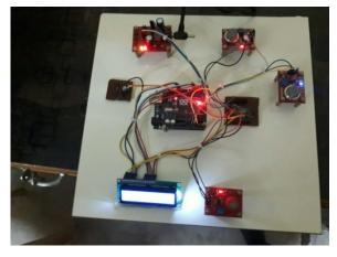
Output: Due to the presence of NO,CO, Nitrite in the exhale breath we detect "asthma diseases" in the person.
