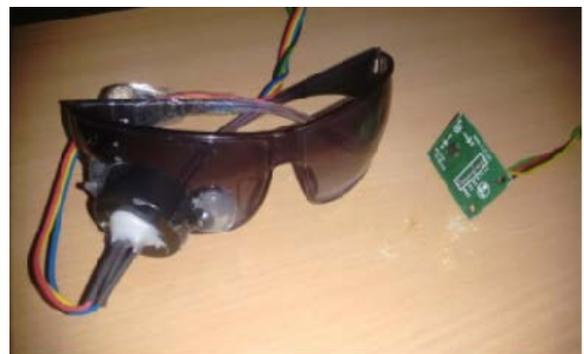
Fig. 10.1 IR Sensor with Accelerometer.
