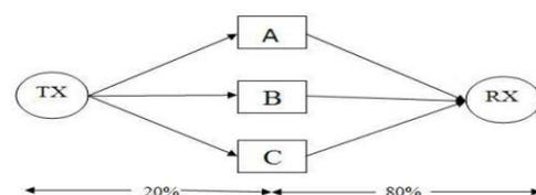
Fig. 1.1 A source node has various candidate nodes which have packet delivery ability for communication of information to the destination node.
