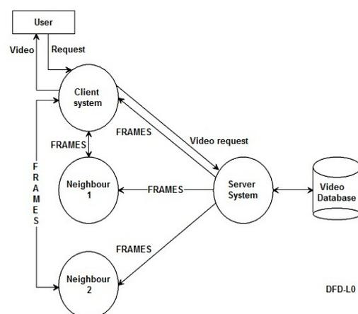
Fig 2.2 Context Analysis diagram depicting the video streaming process.
