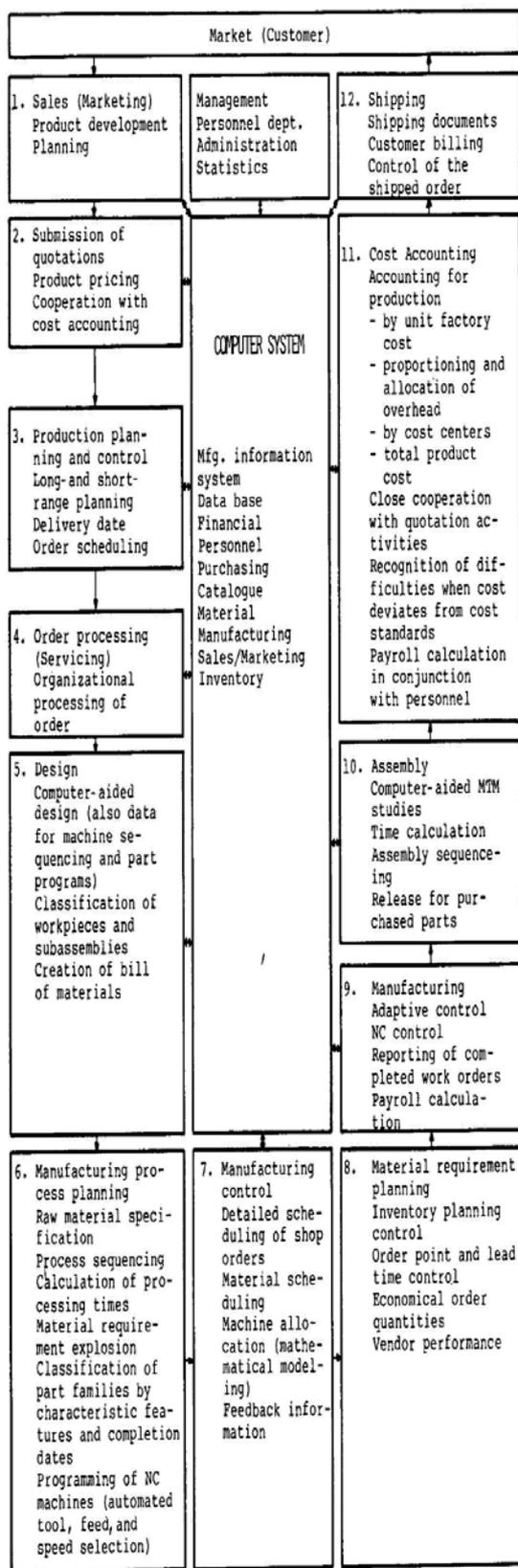
Fig.1. Computer Integrated System Work Flow
