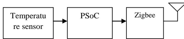
Fig a : Transmitter block diagram
