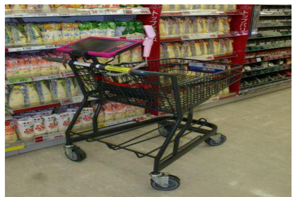
Fig.1: A Trolley is attached with the RFID reader and LCD.
