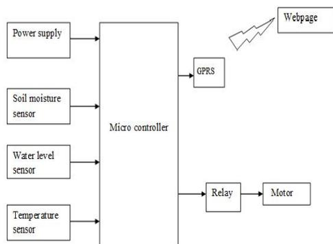
Fig:1 IoT based Auto irrigation System.
