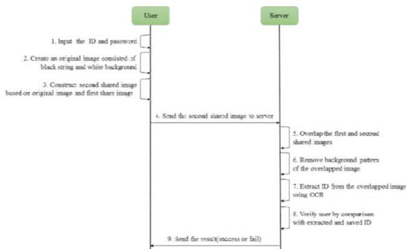
Figure 8. Process of enhanced password Scheme
