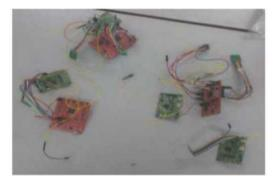
Fig.4: group of wireless sensor nodes
