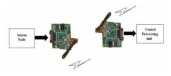
Fig.8: Schematic of peer-to-peer link
