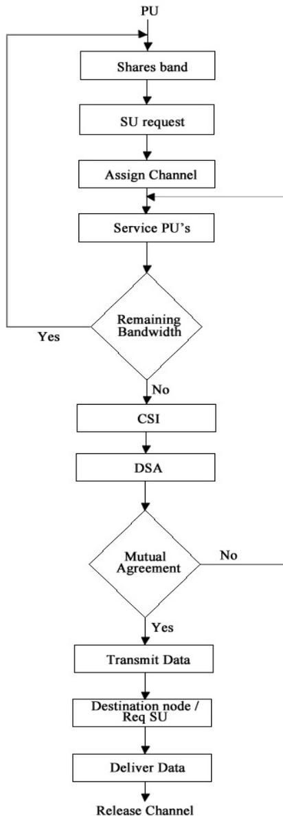
Fig. 5 Multiple channel assignment algorithm
