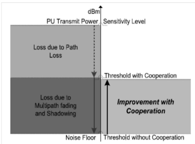
Fig. 4 Sensitivity improvement through cooperative sensing
