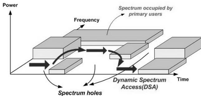
Fig. 2 Spectrum occupied by PU and unoccupied spectrum holes
