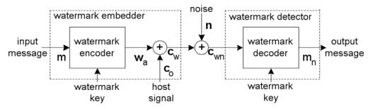
Fig. 2. A steganography system and an equivalent communications model.
