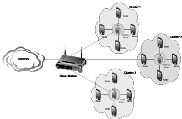
Fig. 3.1 Network Diagram of Proposed Methodology with LEDA-DEEC
