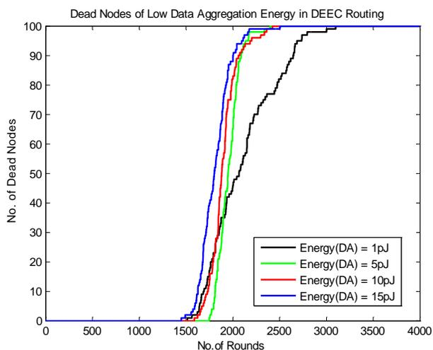
Fig. 4.1 Network life span in terms of dead nodes versus no. of rounds
