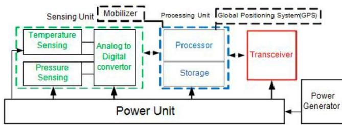
Figure 1.2: Sensor Node's Architecture
