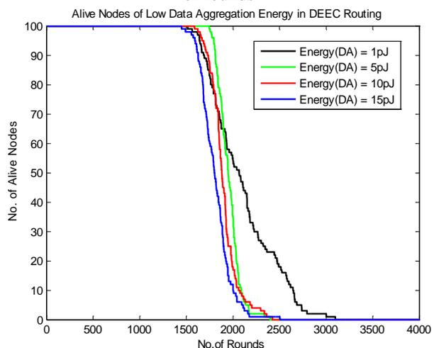
Fig. 4.2 Network life span in terms of alive nodes versus no. of rounds
