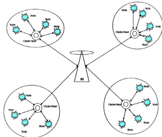
Fig. 2.1. Clustered Architecture Illustrating data aggregation
