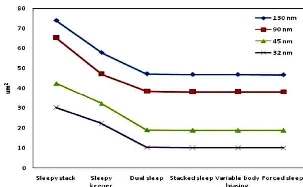
Figure 4.1 shows the area of a chain of four inverters in different technologies. In case of 32 nm technology both the stacked sleep approach and the variable body biasing technique gives -20.31% worst result than the dual sleep approach. Forced sleep approach gives -39% worst results than the dual sleep method.
