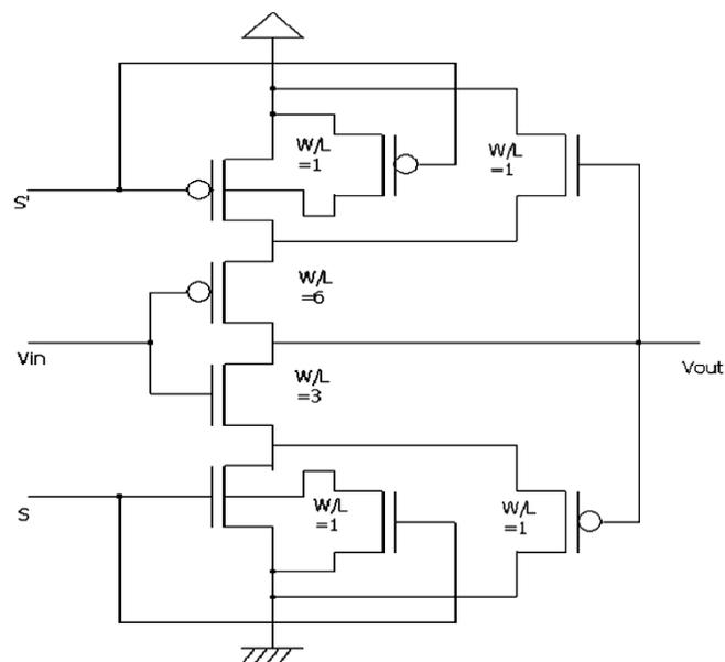
Figure 3.1.1 Structure of variable body biasing technique
