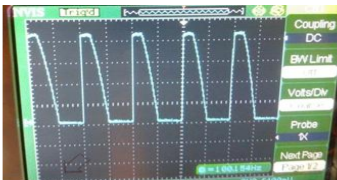
Fig 4.5 Firing angle at 90° forward direction
