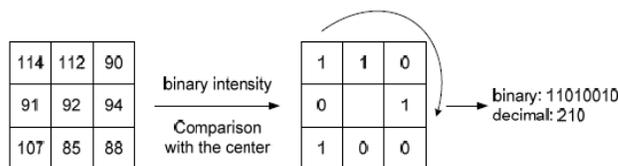
Fig. 1. 2 An illustration of the original LBP calculation.
