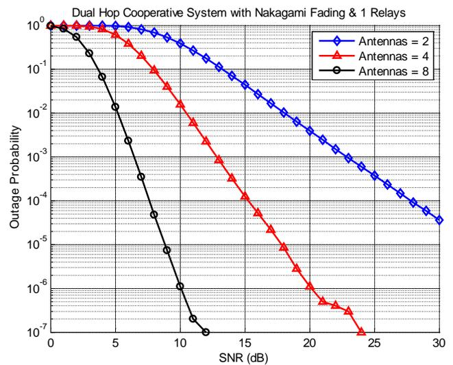
Fig. 4.1 Outage Probability of Dual Hop Cooperative Relay system with multiple antennas and Single Relay
