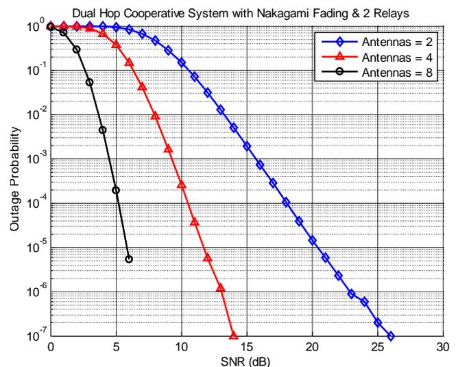
Fig. 4.2 Outage Probability of Dual Hop Cooperative Relay system with multiple antennas and Two Relays
