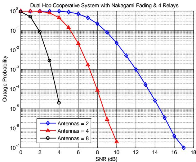
Fig. 4.3 Outage Probability of Dual Hop Cooperative Relay system with multiple antennas and 4 Relays
