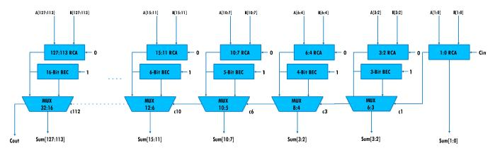
Fig. 5 128-Bit Area, Delay Efficient BEC Based Adder
