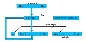
Fig. 4 Two n-Bit Multiplier Design
