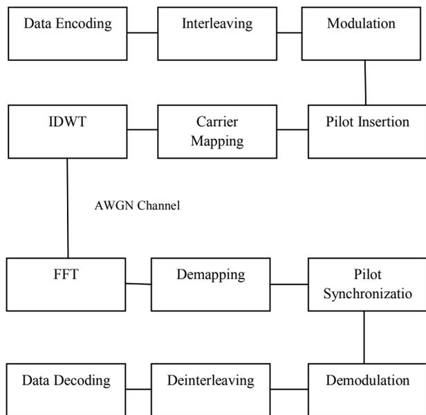
Fig 2. Wavelet based proposed OFDM system design
