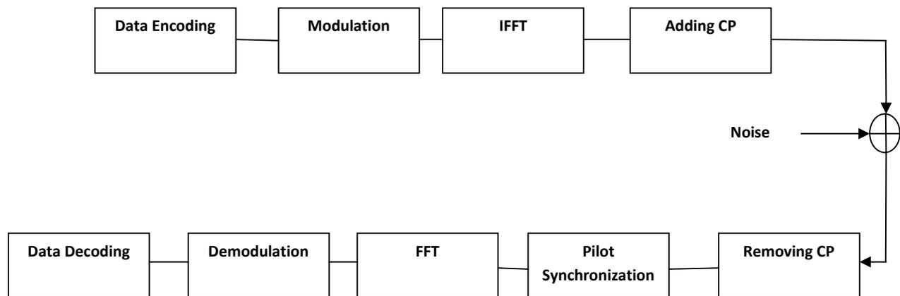
Fig 1. DFT based OFDM transmitter and receiver
