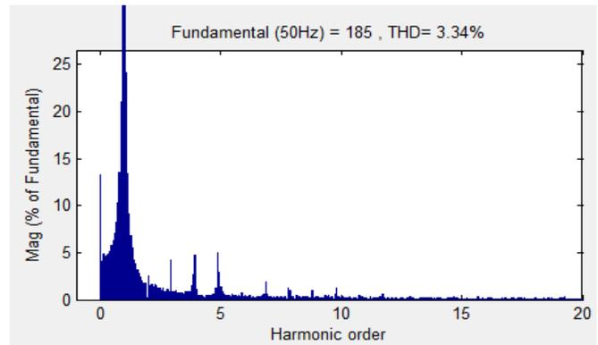
Fig.4.4. THD Analysis of Output Voltage
