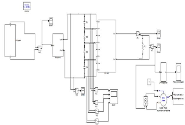
Fig 2 Simulation circuit for 9-level Cascaded Inverter
