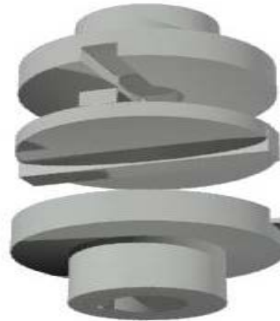
Fig 5.1 model of Oldham's coupling in AutoCAD 3D
