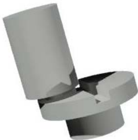
Fig 7.2 AutoCAD model of steel hub with well designed feeder
