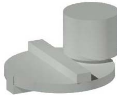
Fig 7.3 AutoCAD model of centre disk with well designed feeder
