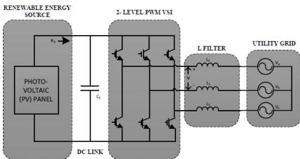
Fig. 1.1. Schematic diagram of Grid Connected PWM Inverter
