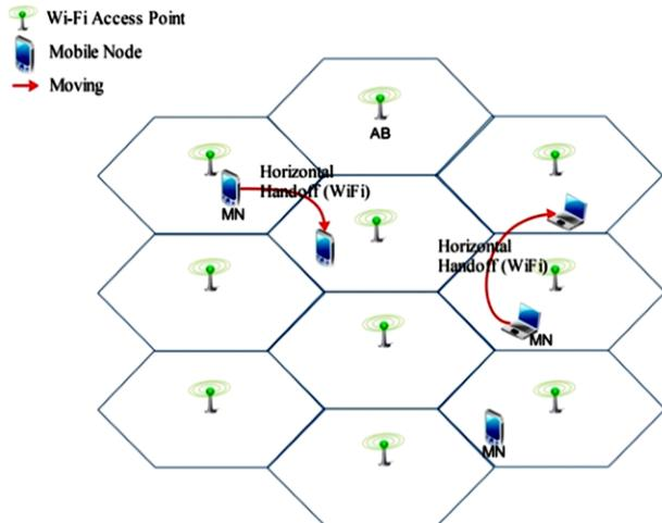
Figure 3: Horizontal handoff (Homogeneous) between Wi-Fi Access Points
