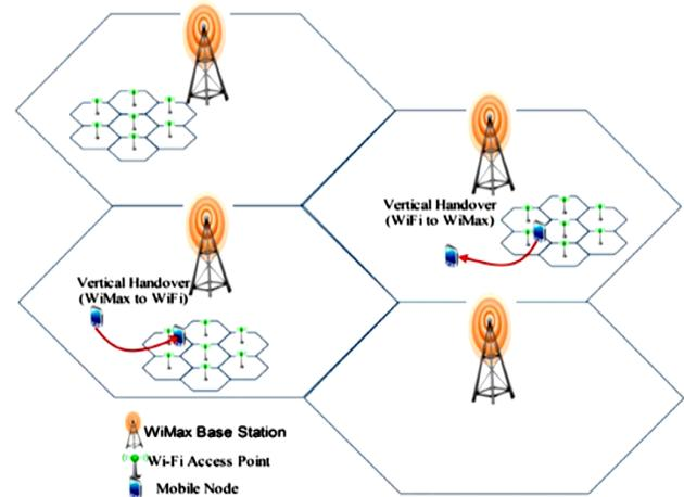
Figure 5: Vertical Handover (Heterogeneous) from Wi-Fi to WiMax and WiMax to Wi-Fi
