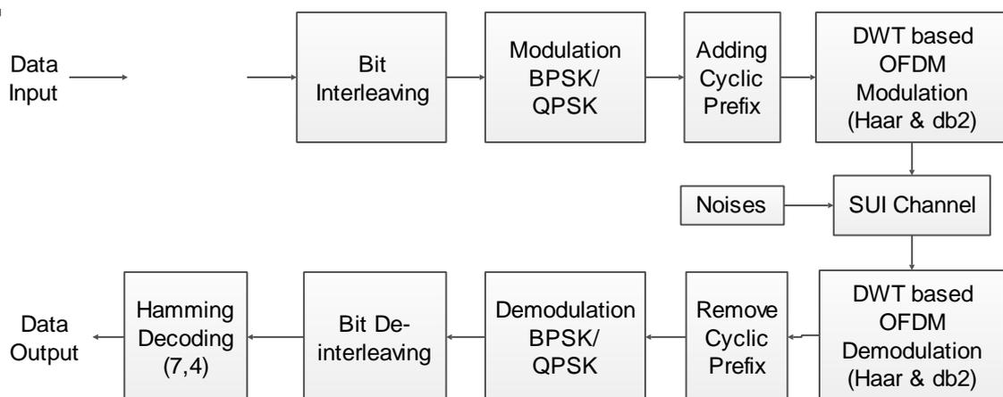
Fig 4.2. Block Diagram of the Proposed Model
