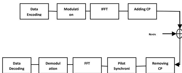
Fig 1.2. DFT based OFDM transmitter and receiver
