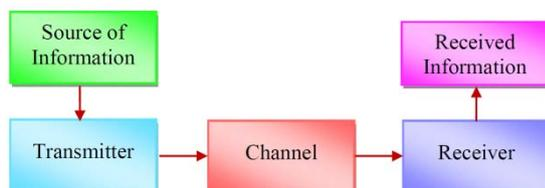
Figure 1.1. A standard digital communication system
