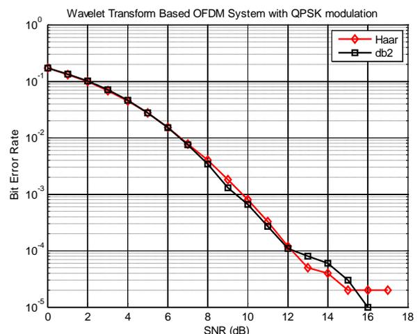
Fig 5.2 Performance outcomes with QPSK Modulation
