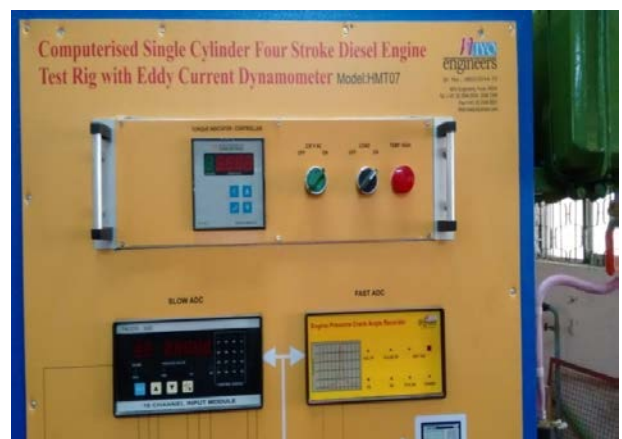
Fig 2.3. Control Panel to apply Load on Dynamometer
