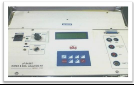
Fig 1-Salinity Measuring Kit [Ref: JADAVPUR UNIVERSITY Pollution Control Lab]
