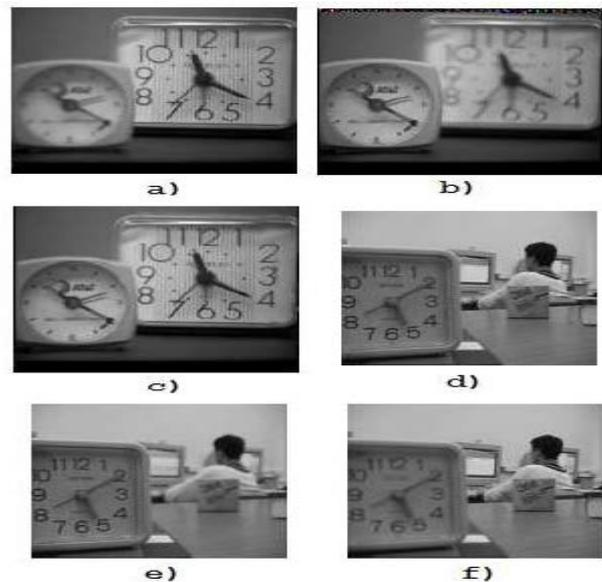
Figure 1: a), b), d), e) Two scene images with different depth of focus, c), f) Fused images
