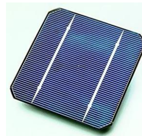
Fig.1.1 A Conventional Crystalline Silicon Solar Cell. Electrical Contacts Made From Bus bars (The Larger Strips) and Fingers (The Smaller Ones) are Printed On The Silicon Wafer
