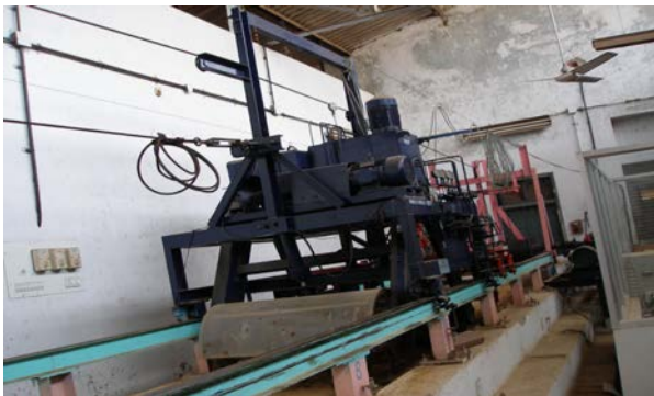
Fig. 3 Test soil bin
