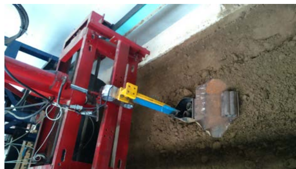
Fig. 2 Test setup with covering device attachment
