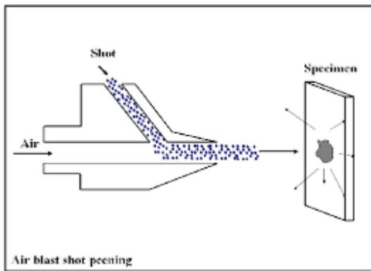
Angle of the impact is too important in the controlled shot peening because it decides the amplitude of the shot struck on the component. In shot peening the as angle increases from 0 to 90 the effect of the shot peening improves and at 90 deg angle the maximum amplitude of impact is attained
