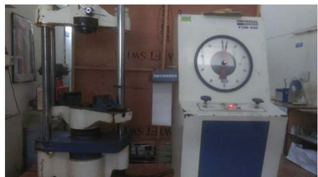
Fig 5.6 Experimental setup for peel off test for Seat Track Assembly
