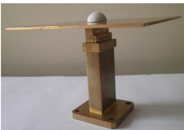
Fig. 2 Photograph of the fabricated rectangular waveguide fed hemispherical DRA using waveguide steps with gd = 100 mm, sl = 10.1 mm, sw = 0.8 mm, st = 1.3 mm, w_1 = 7.0 mm, t_1 = 5.5 mm, w_2 = 4.3 mm, and t_2 = 9.2 mm
