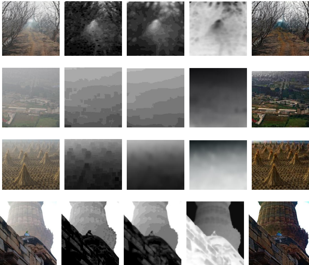
figure 8, 1 st coloum is input image, 2 nd coloum is DCP image, 3 rd coloum is fine DCP with recursive guided filter, 4 th transmission map and last coloum output image
