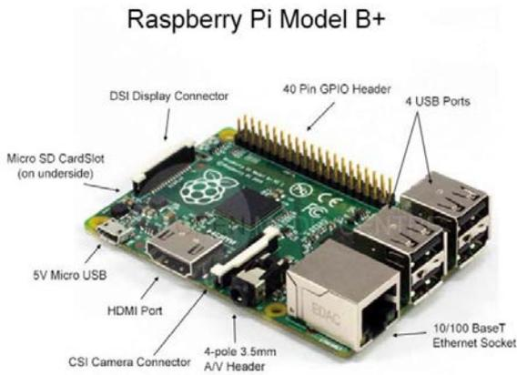
Fig 2. Raspberry pi 2 model b [5]
