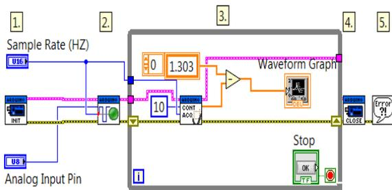
Fig 5.1 showing a VI developed on Lab VIEW to communicate with Arduino.
