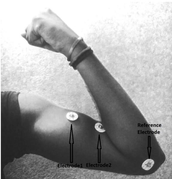
Fig 3.3 Layout of sensor placement. (Bicep muscle)
