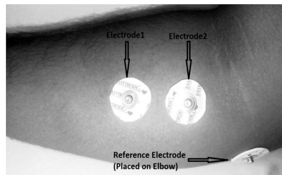
Fig 3.1 Layout of sensor placement.(Forearm Flexor muscles)
