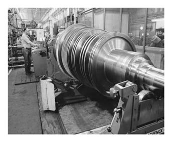
Fig No 1.1 Solid turbine rotor wheels and shaft
