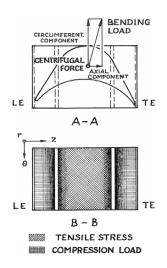
Fig No.2.2 Load and stress distribution due to centrifugal force
