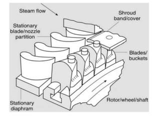
Fig No.1.2 Arrangement of stationary and rotating blades
