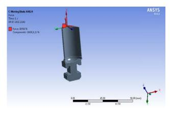
Fig No. 5.4 Centrifugal force acting on blade
