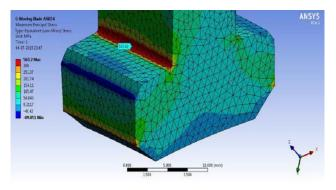
Fig No.5.6 Stress observed in blade
