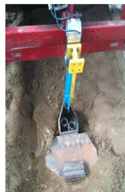
Fig.1 Soil covering attachment with shoe type furrow opener and load
