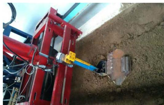
Fig.3. EORT moved with furrow opener and its soil covering attachment
