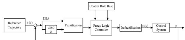
Fig.3.2 Fuzzy control algorithm for substation inspection robot control system
