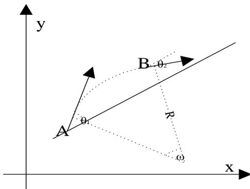
Fig.3.1 Path diagram of substation inspection robot
